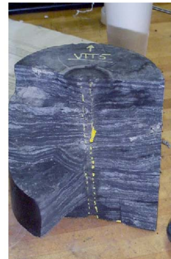
FIGURE SIX Picture Of Shale Cap Rock From Test Five Split Open (Disturbed area is outlined for clarity)
