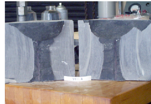
FIGURE NINE Perforation Through The Shale Section – Test Four
