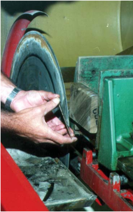
Gene Kullman prepares core for thin slab conventional radiography. With use of the proper technique, it is possible to show enough detail to see the fibers in paper.
