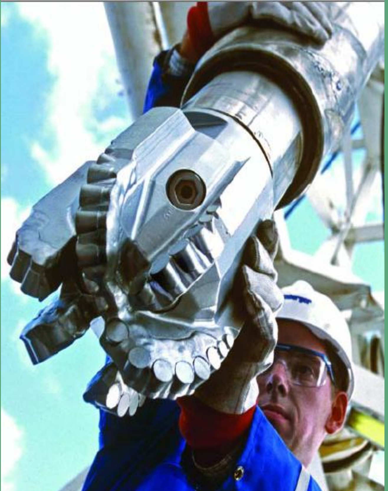
PDC bit on a modern rotary steerable drill system RSD)
