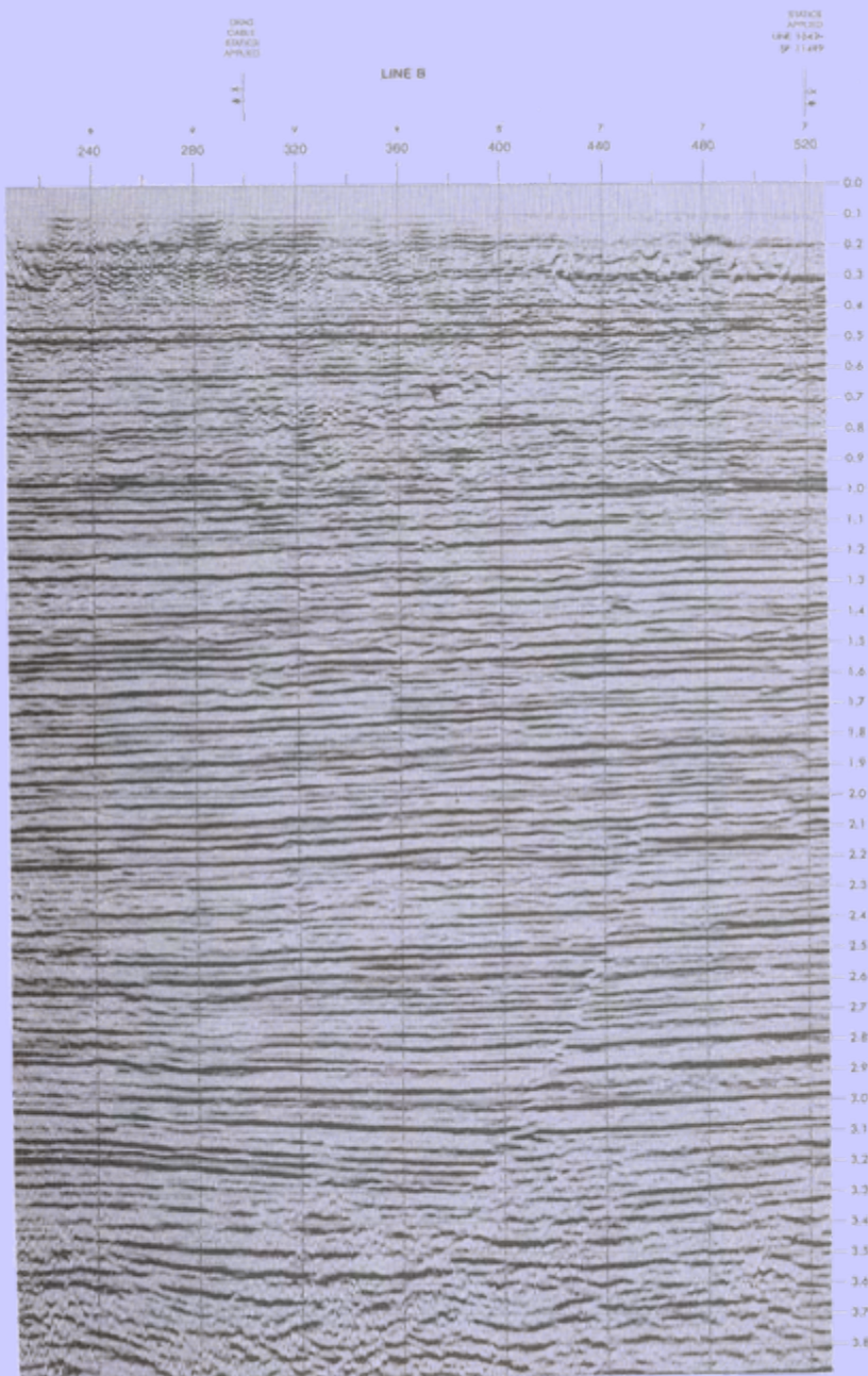
Figure 5-19 Seismic line B. Profile shows gently dipping reflectors cut by a small growth fault. (Seismic data published by permission of TGS/GECO.)
