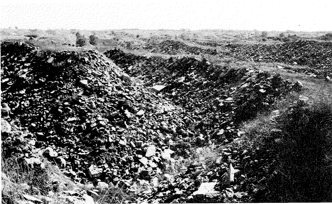
Figure 11. Mined land in the N \frac{1}{2} sec. 3, T. 23 N., R. 17 E., partly reclaimed in accordance with the Oklahoma Mining Lands Reclamation Act of 1968, which required leveling only the tops of spoil ridges to a width of 10 ft. The Iron Post coal was mined at this location between 1968 and June 1971.
