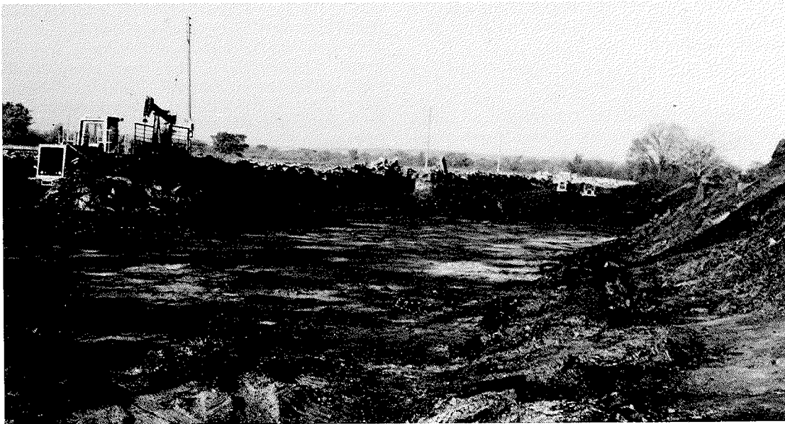
Figure 6. Active strip mine operated (Oct. 1979) by Four D Energy, Inc., in the SE \frac{1}{4} NW \frac{1}{4} NW \frac{1}{4} NE \frac{1}{4} sec. 7, T. 24 N., R. 17 E., Rogers County. Overburden above the Iron Post coal is <10 ft thick at this location. Note small oil-well pump on the "island" at the left (see Appendix 2, measured section 67).
