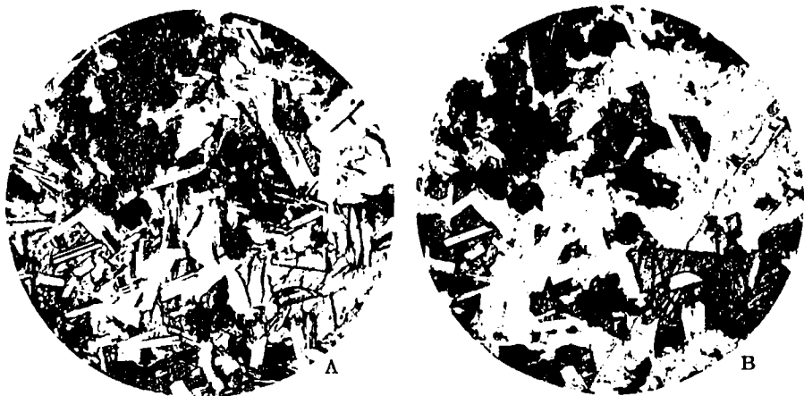
Figure 12. Photomicrographs of diabase.
