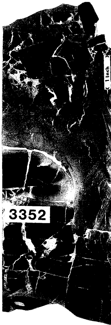
Figure 3. Crackle-brecciated rock subjacent to an intra-Arbuckle disconformity. Many fractures are enlarged and filled with micritic sediment. (Oliphant-Lafortune core, -3,352 ft.)
