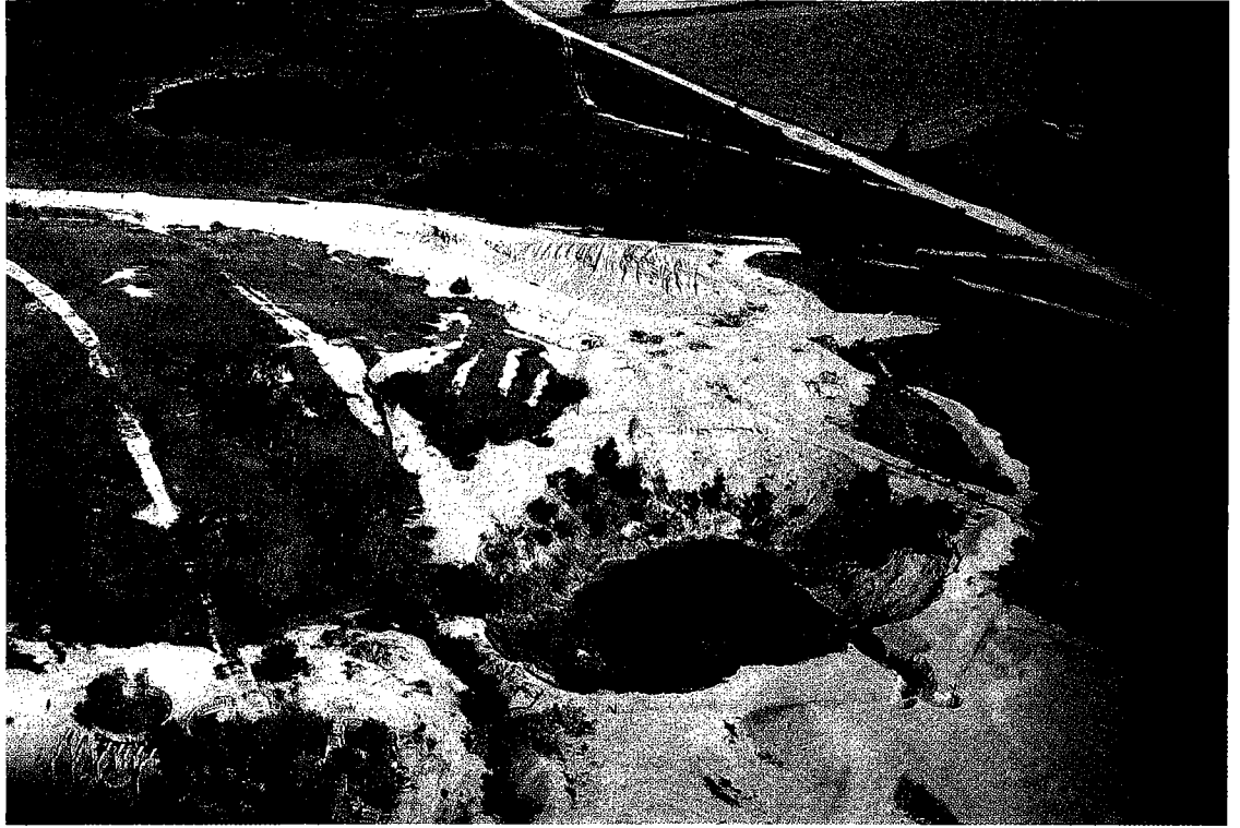
Figure 13. Two major shaft-related collapses, Anna Beaver lease, 29N-23E-19 (6, upper; 7, lower).
