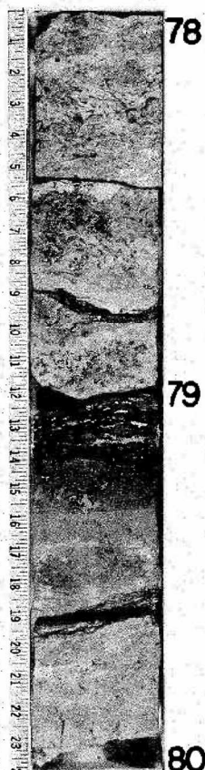
Figure 7. Part of the lower Altamont Member with a well-developed dark-gray algal shale (at 79'). Triangular inclusions in algal shale are cross sections of branches of the common bryozoan Prismopora triangularis .
