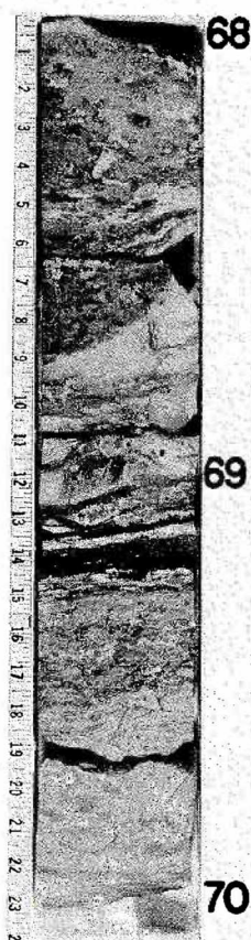
Figure 6. Typical lithology in Altamont Limestone Member. Section of core shown consists of alternating beds of limestone and algal shale. Limestone is mainly dense uniform medium light-gray calcisiltite containing blades and flakes of algae replaced by brown sparry calcite. Algal shale is medium dark gray with a faint olive tinge. It occurs in fine wavy laminae containing pods and lenses of coarse crinoidal sand. At 69 feet is a 2-inch lump of fine calcarenite enclosed in algal shale.
