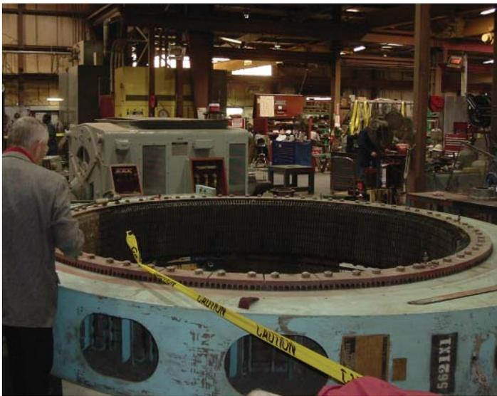
Figure 3. OKAA field trip at Evans Enterprises. Giant motor being repaired is from an OKAA member manufacturing plant's ball mill. (Photograph by Stan Krukowski, OGS.)
