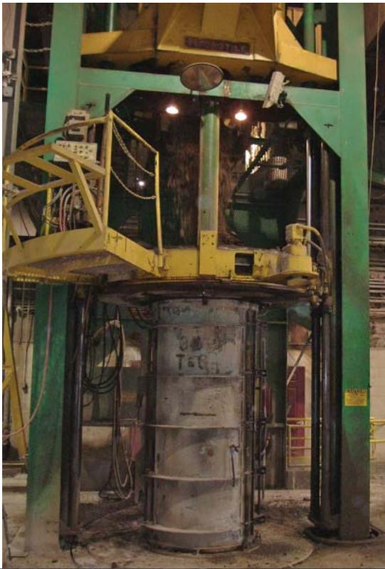
Figure 1d. *Steel concrete pipe mold prior to injection and rotation of concrete. (Photograph by Stan Krukowski, OGS.)*
