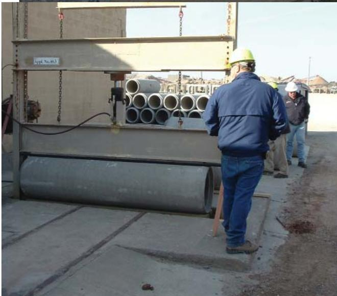
Figure 2. *Hanson Pipe and Precast LLC plant in Oklahoma City. Concrete pipe is undergoing pressure testing to meet ASTM standards. (Photograph by Stan Krukowski, OGS.)*
