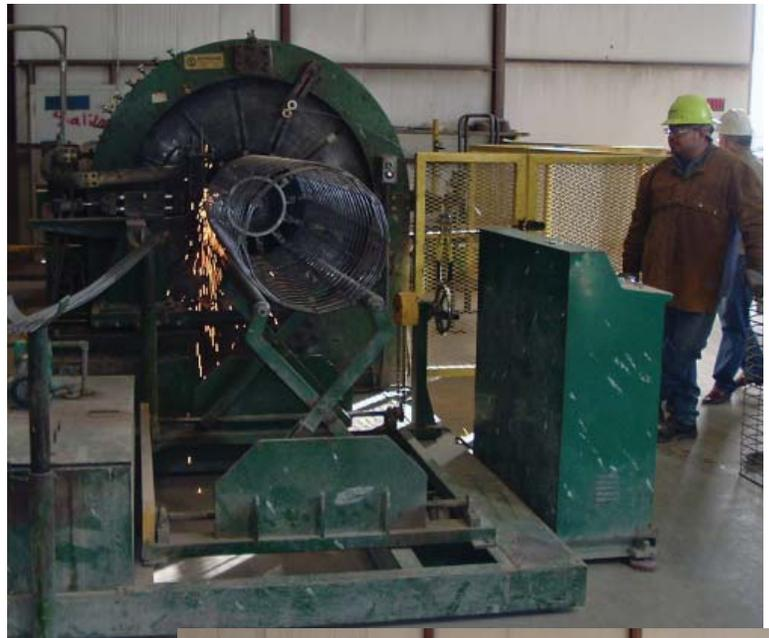
Figure 1b. Finished reinforced steel cage for concrete pipe manufacture. (Photograph by Stan Krukowski, OGS.)
