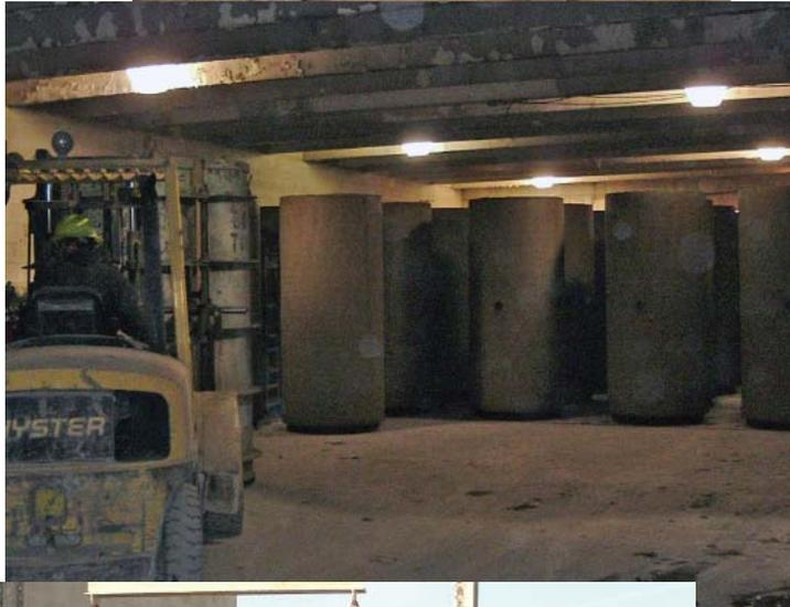
Figure 1f. *Concrete pipe undergoing drying and setting in drying warehouse sauna at 60°C and 100% relative humidity. (Photograph by Stan Krukowski, OGS.)*
