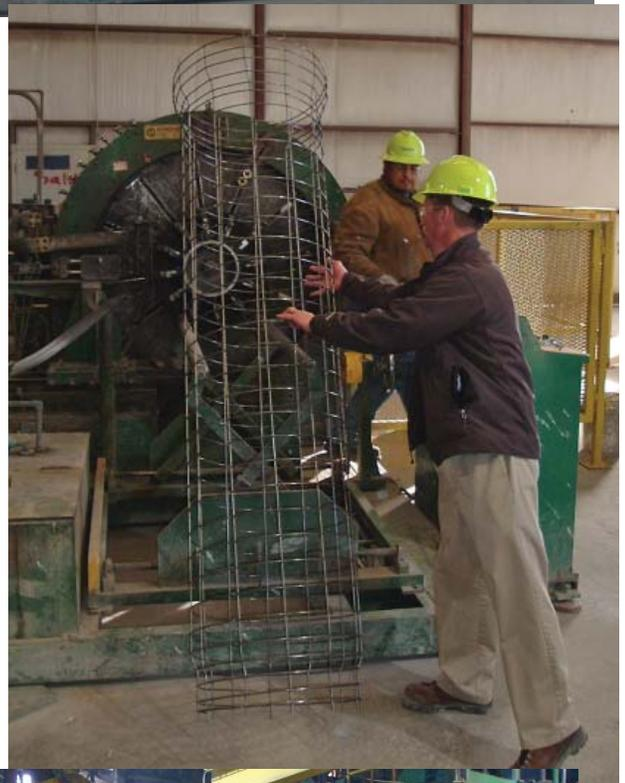
Figure 1c. Hanson Pipe and Precast tour guide explaining manufacture of concrete box culvert. Foreground: steel reinforced cage prior to concrete injection; background: finished concrete box culvert. (Photograph by Stan Krukowski, OGS.)
