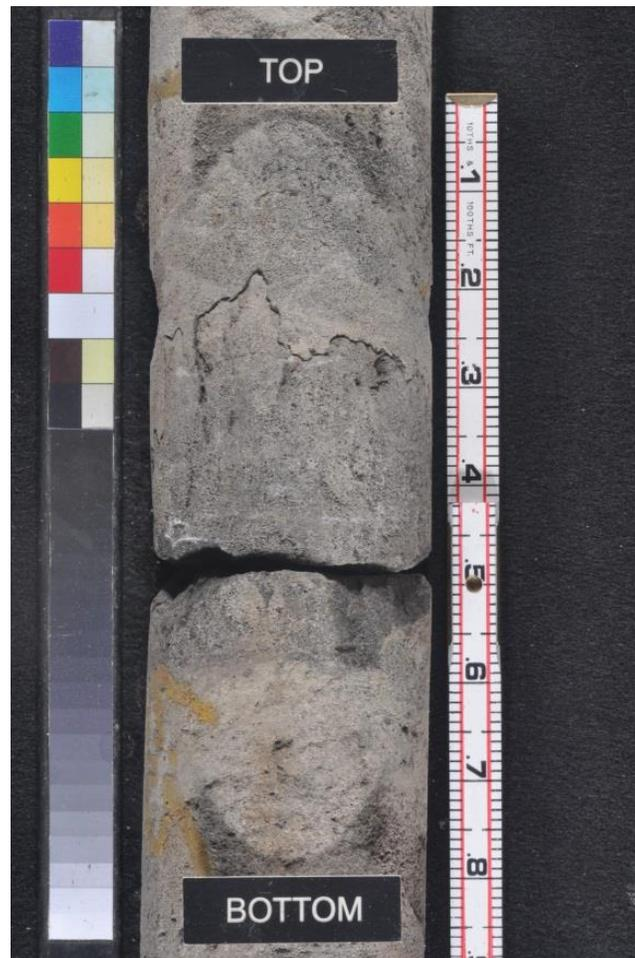
Figure 4 Dry Wedgewood Biddle-Burke – 6 Core from 3365 to 3365.9 ft, showing a porous carbonate section with a visible stylolite
