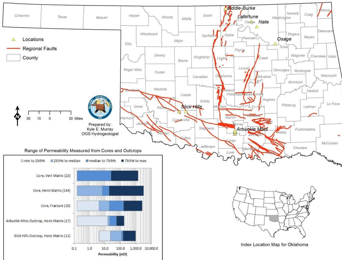
Figure 1 Map showing locations of Arbuckle cores and outcrops examined in this study, with chart for various permeability measurements of cores and outcrops.
