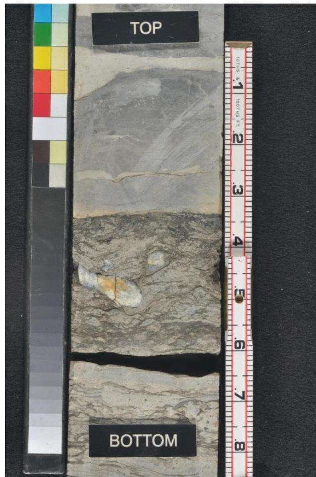
Figure 2 Dry Oliphant LaFortune – 3 Core from 3334–3335 ft, showing the contact of the overlying Simpson Group with the underlying Arbuckle Group at about 0.35 ft on the measuring tape
