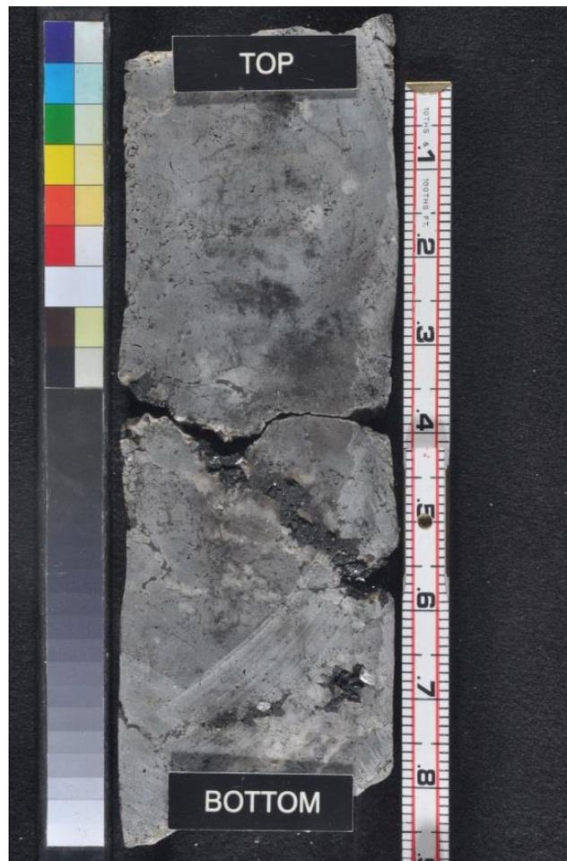
Figure 3 Dry Oliphant Nate - 1 Core from 2862.2 to 2862.9 ft, showing a bituminous vein with apparent fracturing and vuggy porosity
