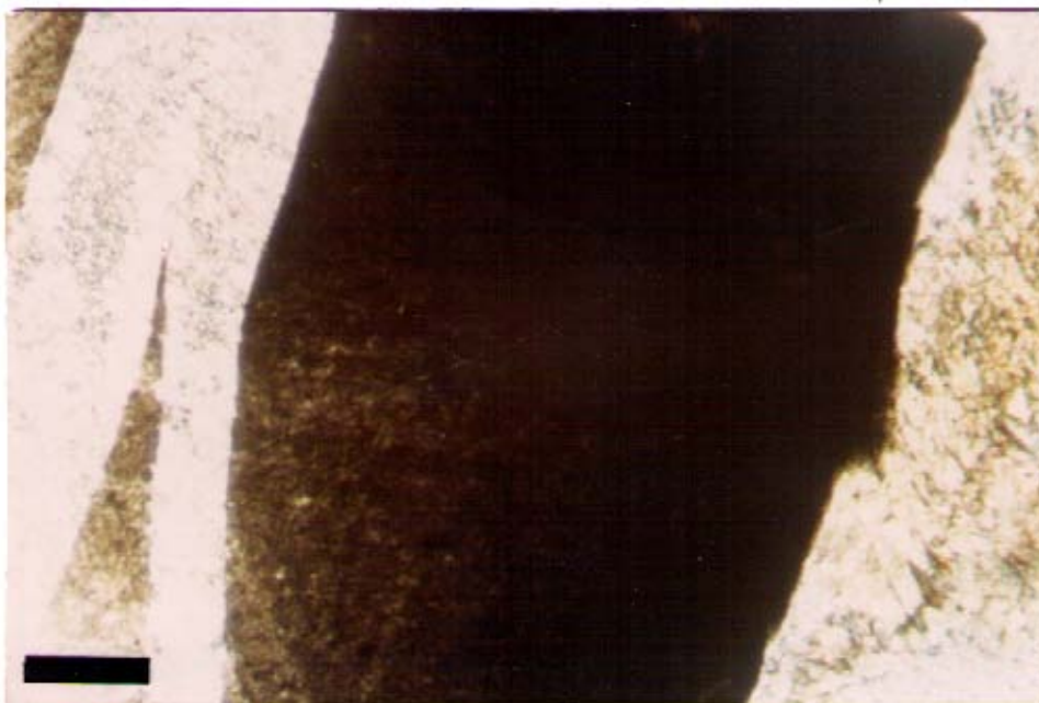
PLATE 10: Dark gray graphitic slate cut by chalcedony filled fractures. Collier fm., 350-60'.
