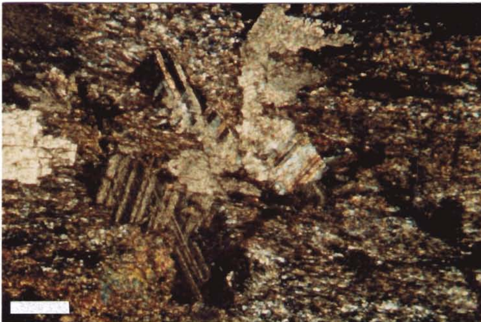
PLATE 15: Metamorphosed dolomite crystals in talc schist. Collier fm., 650-60'.
