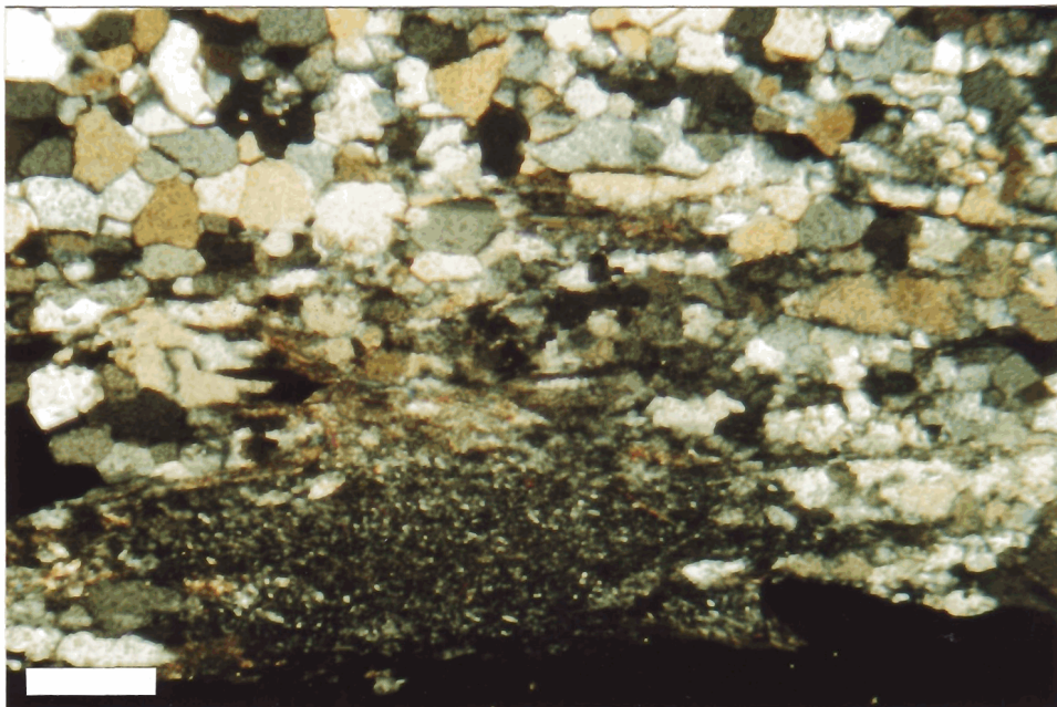
PLATE 126: Mica partings in schistose quartzite. Trace rutile needles and chert (bottom center). Womble fm., 11,160-70'.
