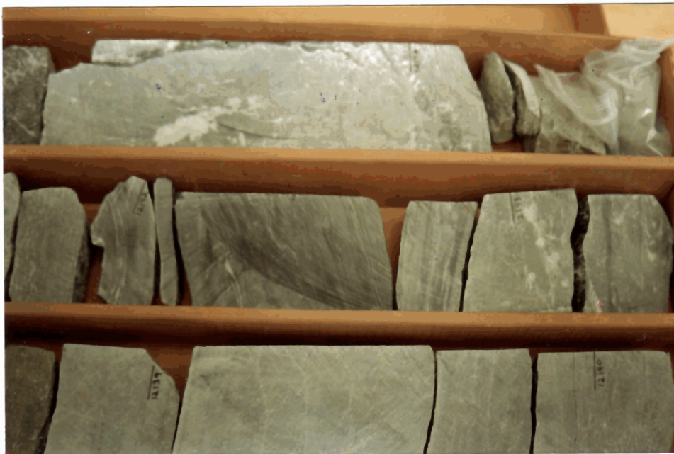
PLATE 263: Core #1 (slab) bottom 12,138-40', center 12,141-43', top 12,145-47'. Stylolite cut sandy micaceous marble.
