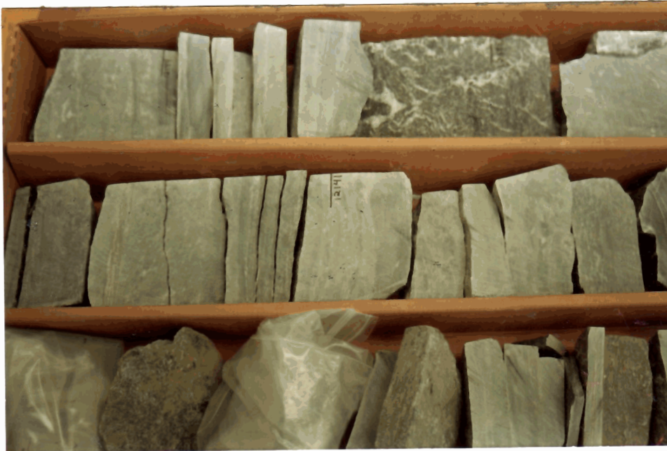
PLATE 262: Core #1 (slab) bottom 12,137-38', center 12,140-41', top 12,144-45'. Brecciated and stylolite cut sandy micaceous marble.
