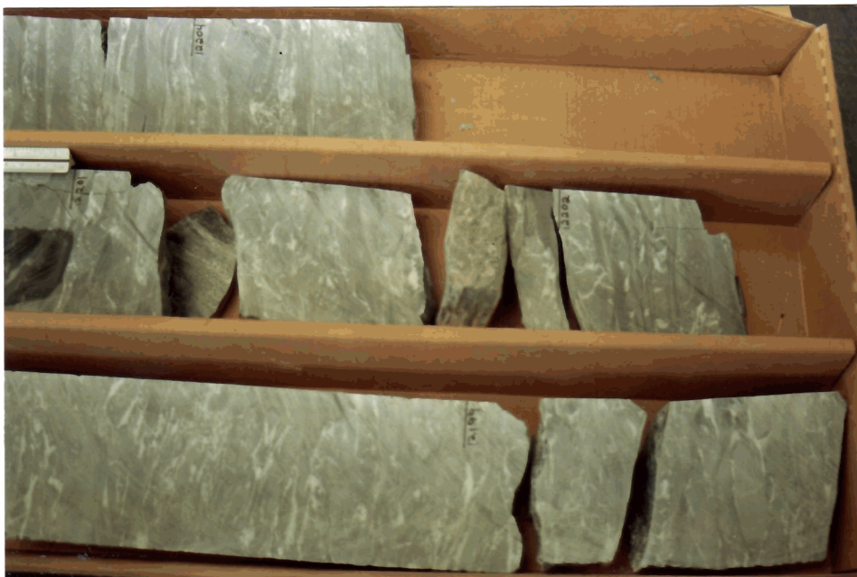
PLATE 297: Core #2 (slab) bottom 12,198-99', center 12,201-02', top 12,204'. Soft sediment deformed, becciated and stylolite cut meta-dolomite.
