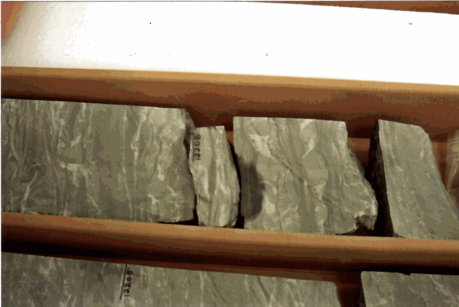
PLATE 307: Core #2 (slab) 12,207-08'. Soft sediment deformation and rip-up cast in meta-dolomite cut by numerous thick stylolites.
