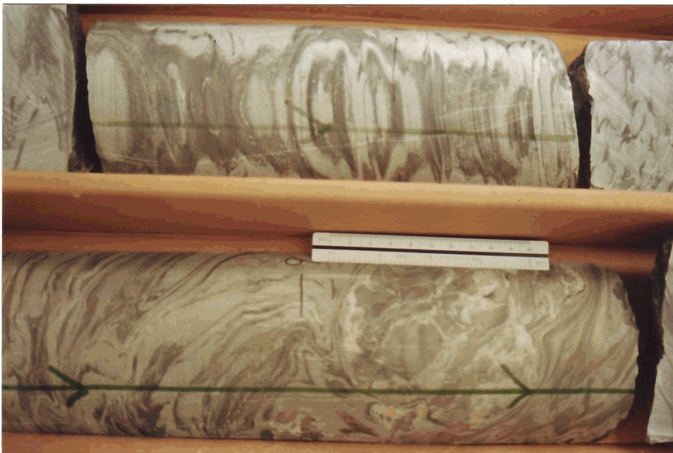
PLATE 275: Core #2 (slab - outside surface) bottom 12,158', top 12,161'
