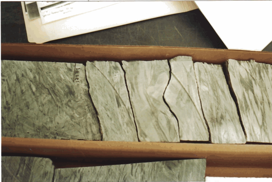
PLATE 282: Core #2 (slab) 12,171'. Note at 12,171' and above the core appears to represent soft sediment deformation, while below 12,171' the core appears to exemplify extensive tectonic deformation.
