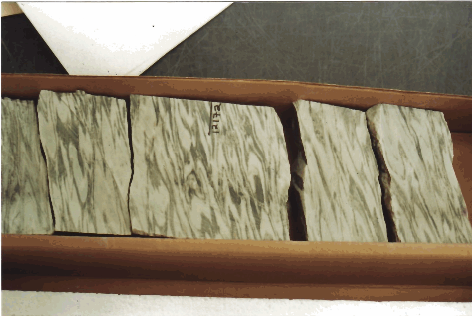
PLATE 283: Core #2 (slab) 12,172. Extensive tectonic deformation in marble.
