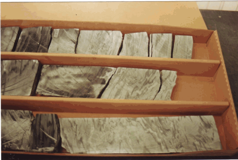
PLATE 273: Core #2 (slab) bottom 12,158-60', center 12,161-62', top 12,164-65'. Tectonically deformed sandy marble.
