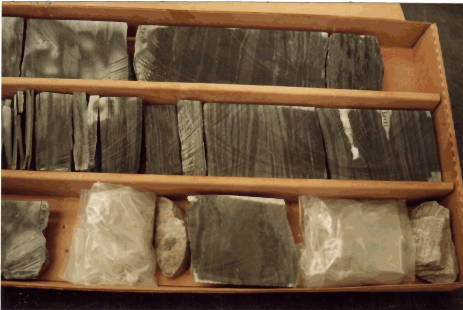
PLATE 267: Core #2 (slab) bottom 12,150-51', center 12,152-54', top 12,155-56'. Extensive stylolite development (dark) in sandy marble.
