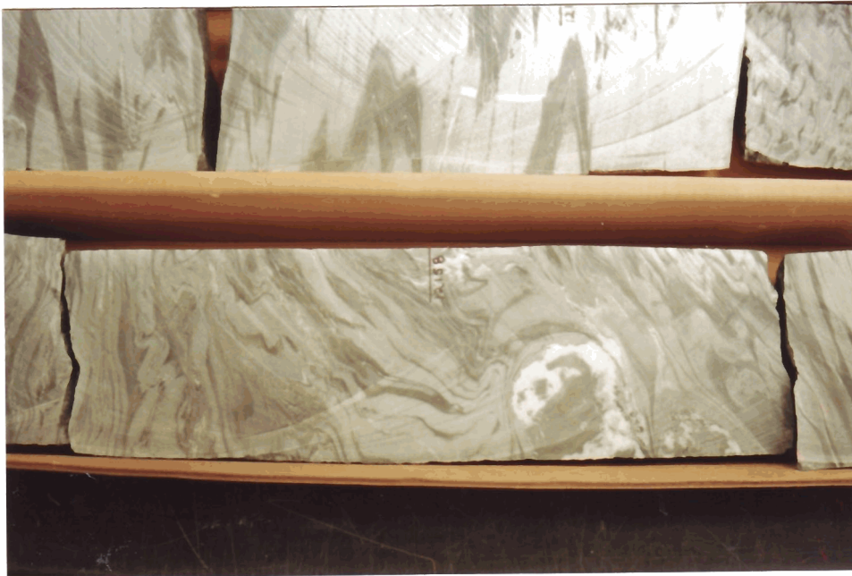
PLATE 274: Core #2 (slab) 12,158' and 12,161'. Note what appears to be soft sediment deformation at 12,158' and definite compressive folding at 12,161'.
