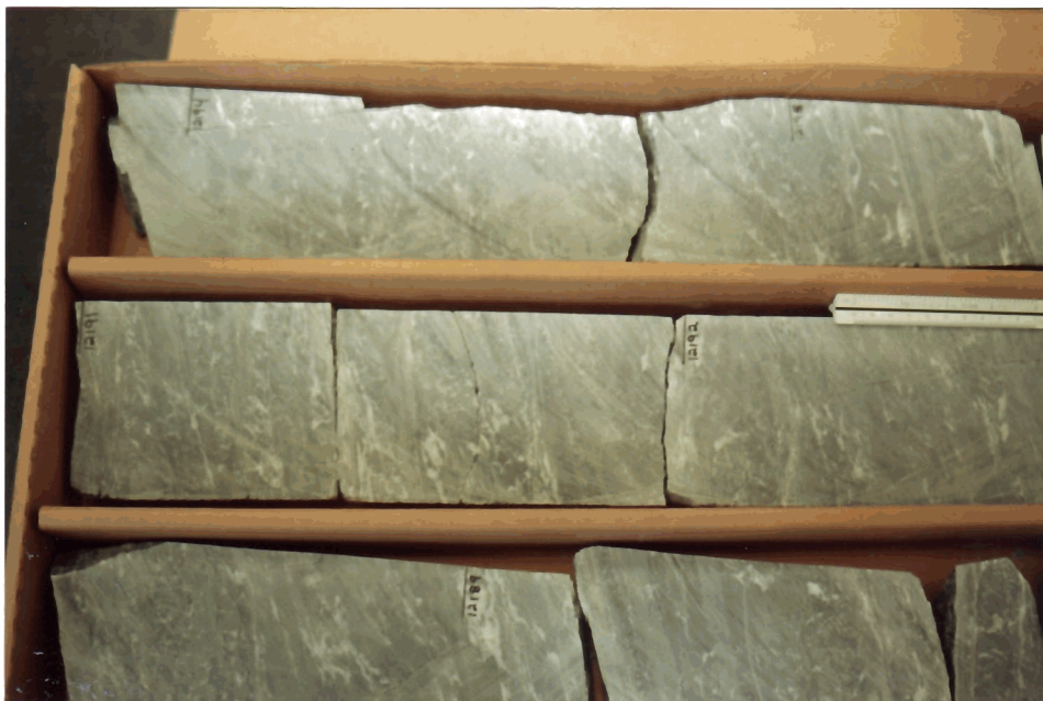
PLATE 292: Core #2 (slab) bottom 12,188-90', center 12,191-92', top 12,194-95'. Brecciated and stylolite cut meta-dolomite.
