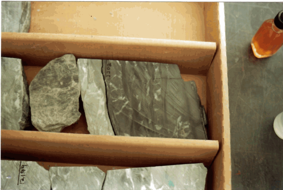
PLATE 303: Core #2 (slab) 12,202'. Soft sediment deformation and rip-up cast in meta-dolomite. Note several horizontal stylolites which contain graphitic micaceous dolomite. Brecciated, stylolite cut and rip-up cast in meta-dolomite..
