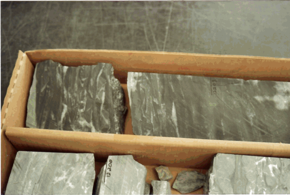
PLATE 300: Core #2 (slab) 12,202-03'. Brecciated meta-dolomite with extensive stylolite development.
