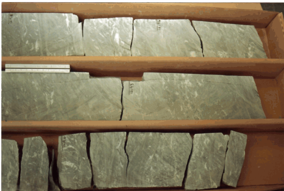
PLATE 293: Core #2 (slab) bottom 12,190-91', center 12,192-93', top 12,195-96'. Brecciated and stylolite cut meta-dolomite. At 12,190' rip-up cast.
