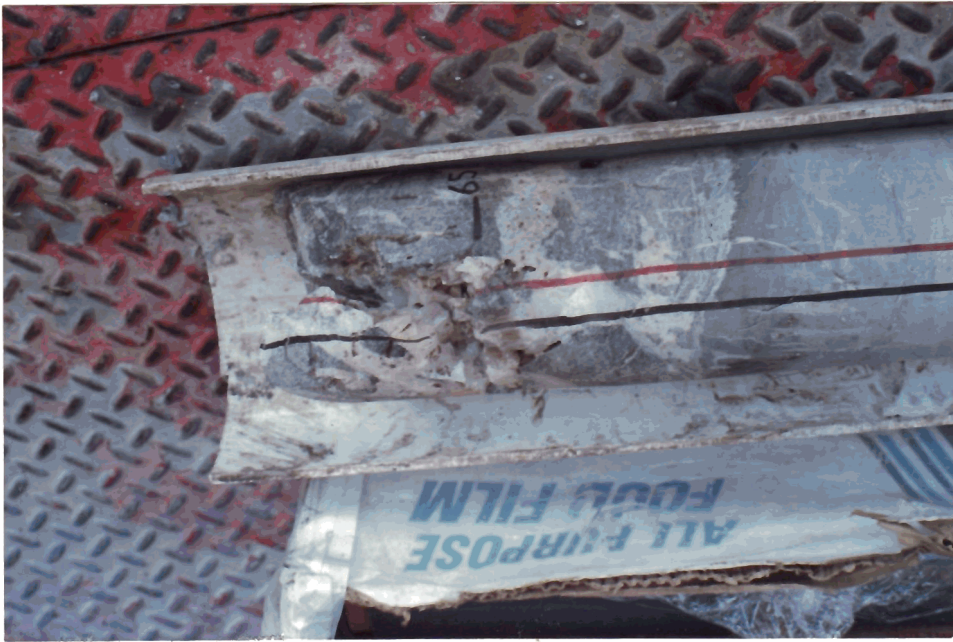
PLATE 317: Core #3 "65" equals 14,265'. Note large vuggy porosity in fracture which also shows large quartz and calcite crystals growing in fracture.
