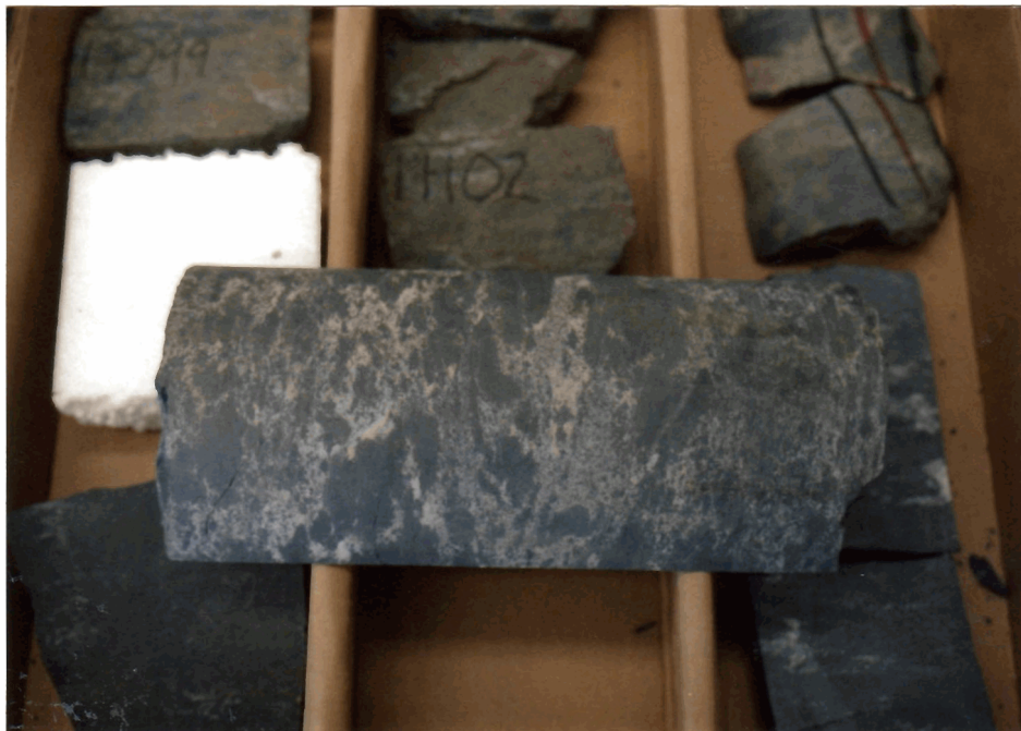
PLATE 362: Core #4 (slab) 17,102'. Brecciated graphitic meta-dolomite.
