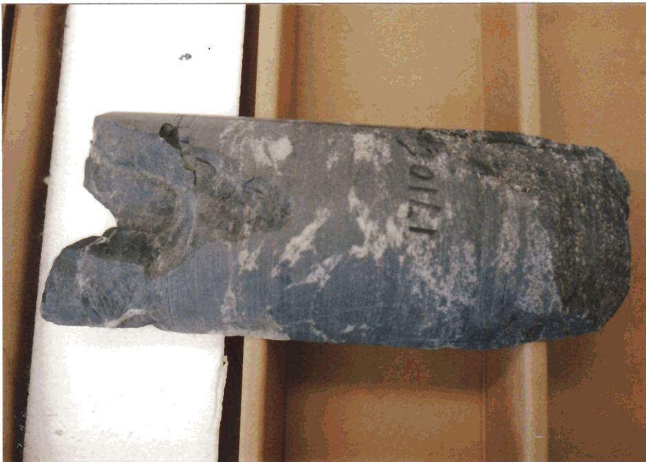
PLATE 369: Core #4 (slab) outside surface 17,105'. Brecciated meta-dolomite and phyllite.
