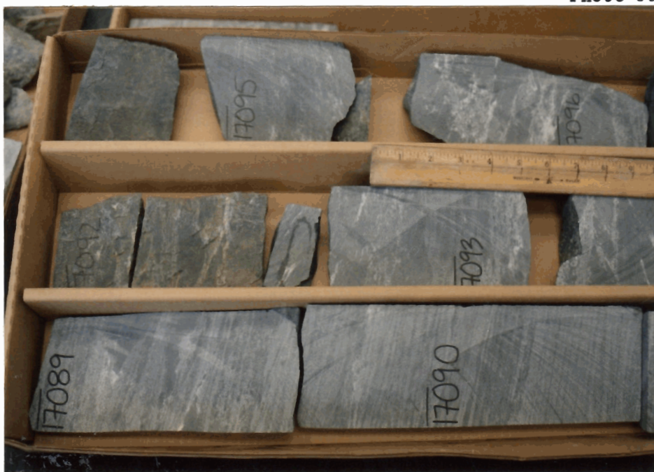
PLATE 352: Core #4 (slab) bottom 17,089-90', center 17092-93', top 17,095-96'.
