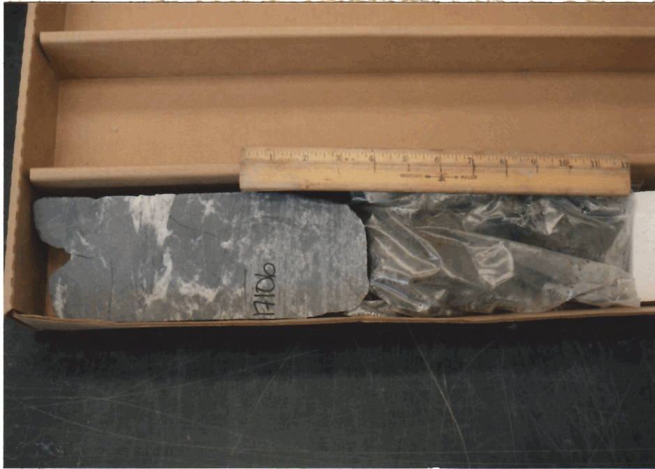
PLATE 370: Core #4 (slab) 17,106'. Fractured stylolite cut phyllite and meta-dolomite.
