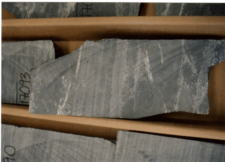
PLATE 355: Core #4 (slab) 17,093'. Parallel bedded stylolite above strongly tectonically deformed phyllite and meta-dolomite.
