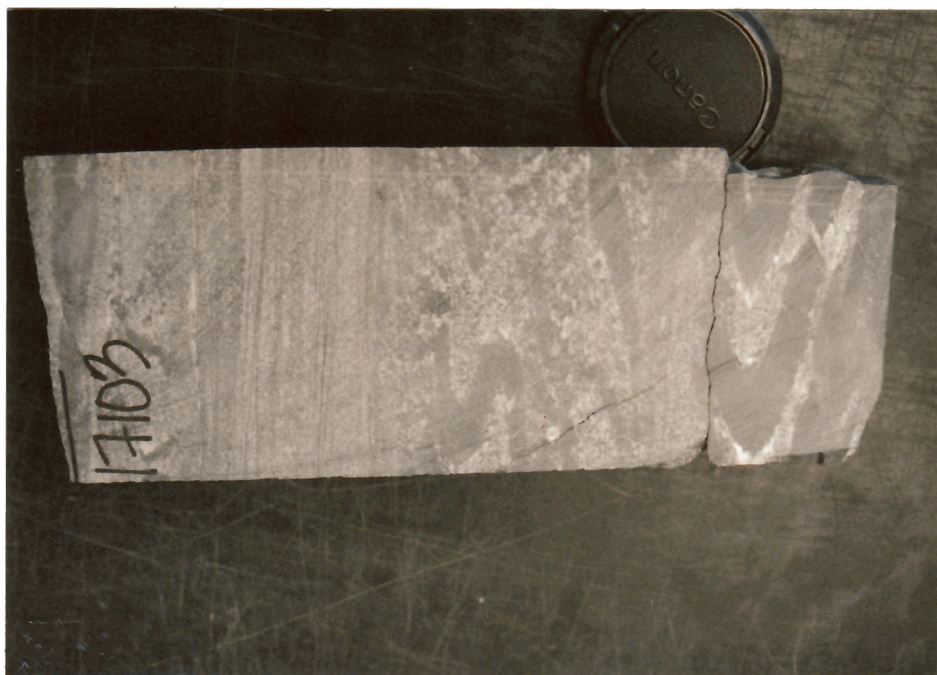
PLATE 363: Core #4 (slab) 17,103'. Large horizontal stylolite in very tectonically deformed phyllite and meta-dolomite.
